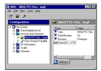
Click on the plus sign next to **Devices and Interfaces** to reveal a list of your installed IMAQ devices.
